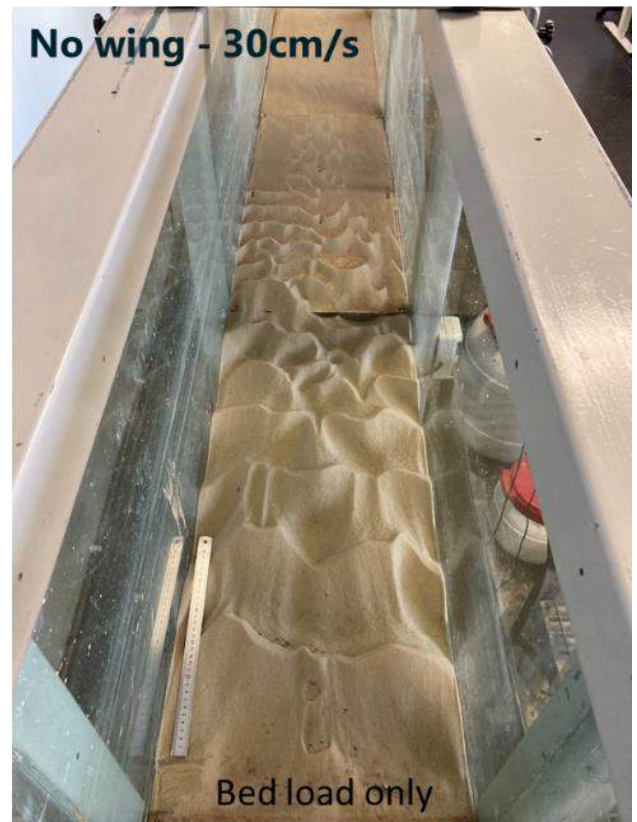
Figure 1: Flume experiments of the Sand Wing with mobile sand bed. Left: Sand Wing with 30° orientation; Right: no Sand Wing. Both experiments were performed with 0.3 m/s flow velocity.
