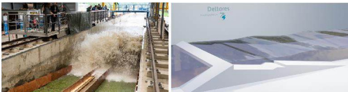
Figure 1: Wide Green Dike under wave attack. Left: Physical flume. Right: Numerical flume.
