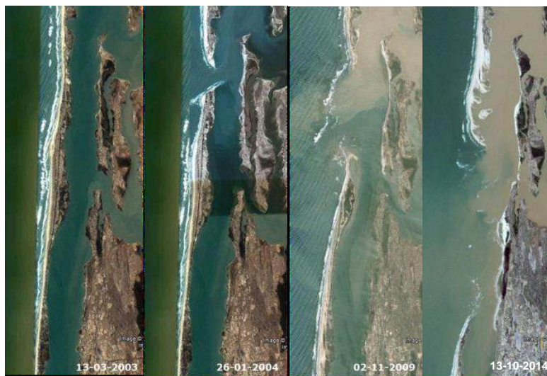
Figure 1: The Langue de Barbarie sandspit in Senegal just before, and the years following, the creation of the artificial breach (Source: Google Earth).
